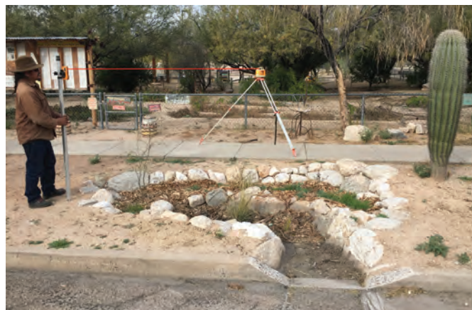
Fig. A1.11D. Omar is measuring the elevation of the rain garden's top zone on its downstream side. Ideally, this point should be at least 4 inches (10 cm) higher than the curb cut inlet of the eddy basin shown here (or the curb cut outlet of a flow through basin ) to ensure that water will not overflow and erode the dirt pathway.
