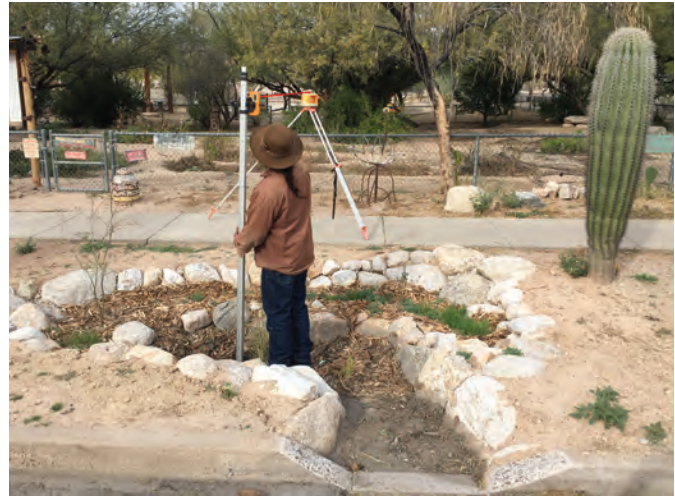
Fig. A1.11B. Next, Omar is taking an elevation measurement at the bottom of the infiltration basin. The deeper the basin bottom is in relation to the curb cut inlet, the greater the basin’s water-harvesting capacity. If the basin bottom is higher than the inlet, it won’t work.
