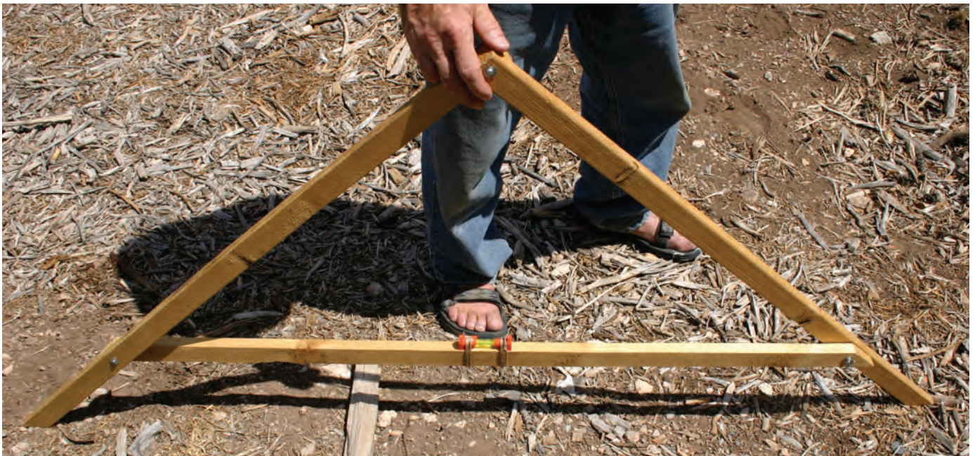
Fig. A1.10. Chris Meuli’s line-level A-frame. A bubble level tool is lashed to horizontal bar (look below Chris’ toes). Chris bolts his A-frame together with wing nuts so he can disassemble and fold it up for easy storage. His A-frame is only as tall as his waist, which allows him to use the tool under the branches of trees.
