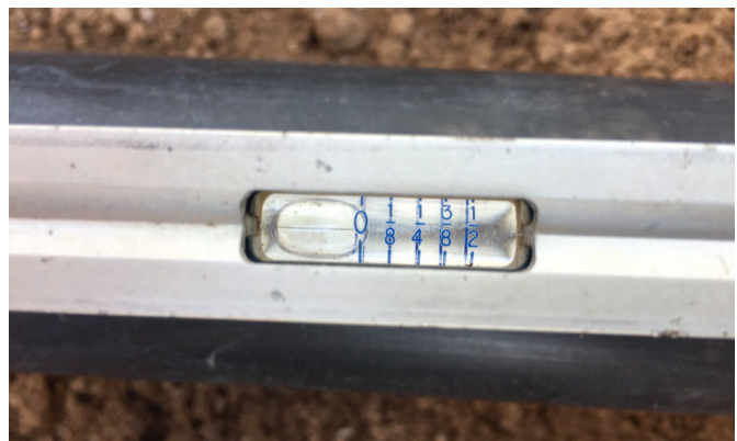
Fig. A1.14C. Tool Box Level with its grooved side up and its magnetic side down. Vari-Pitch vial has been turned so slope measurements can be read from above. Here it reads level. Note how the edge of the bubble in the vial touches and reads “0.”
