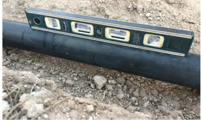
Fig. A1.14A. 12-inch Empire Magnetic Tool Box Level positioned with magnet side up and grooved side down to fit on the pipe, so slope measurements can be read from the side of the level. See fig. A1.14B for close up.
