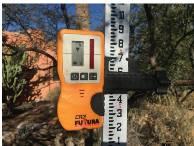
Fig. A1.12. The arrow on the laser receiver's display signifies that the receiver must be moved down to become level with the laser transmitter. As needed, you can slide the receiver itself up or down on the measuring rod, or slide the adjustable section of the measuring rod up or down; or move the base of the measuring rod to a higher or lower point in the landscape if you are trying to find a point that is level with a section of the landscape previously measured.
