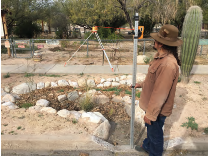
Fig. A1.11A. Omar is using a laser level to take an elevation measurement at the curb cut inlet of a street-side rain garden's water-harvesting basin. This is the reference elevation: we want to know how much higher or lower all other points are in relationship to this point where water will enter the basin.
