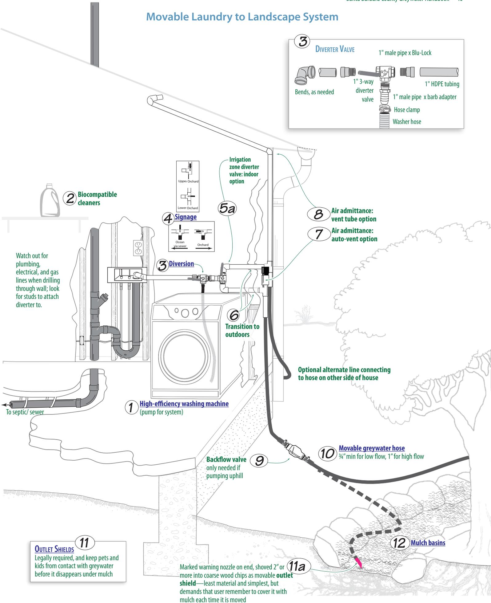
Marked warning nozzle on end, shoved 2" or more into coarse wood chips as movable **outlet shield**—least material and simplest, but demands that user remember to cover it with mulch each time it is moved
