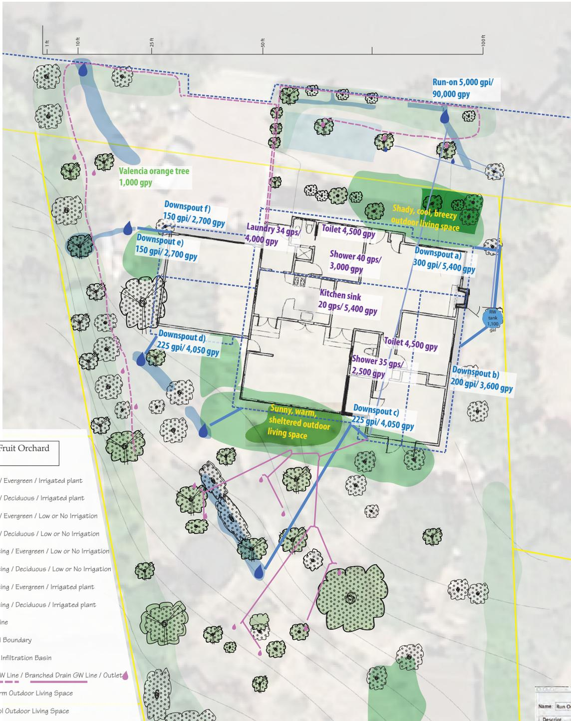
Sample Site Plan, based on a lightened Google Earth image, showing greywater sources and quantities, rooftop rainwater sources and quantities, and irrigation need.
