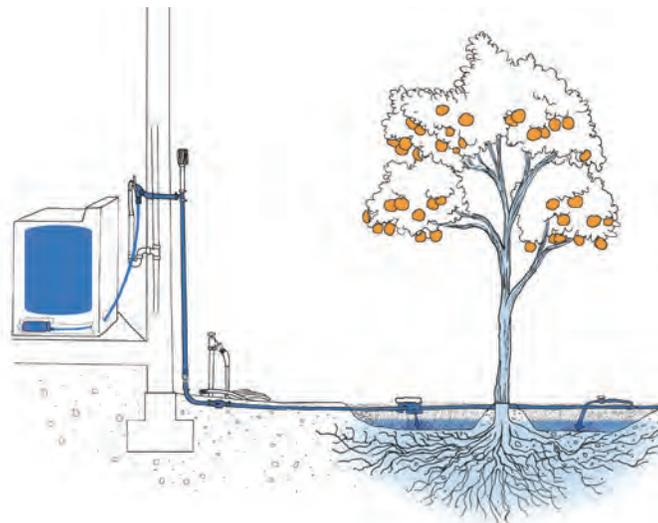
Laundry greywater is the easiest and most common greywater source to reuse for irrigation.
