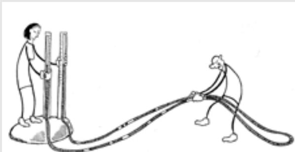
Fig. A1.3. Removing air bubbles from tubing
